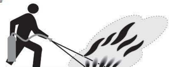
3. Extinguish by squeezing the lever a number of times. Do not empty the extinguisher all at one time.
